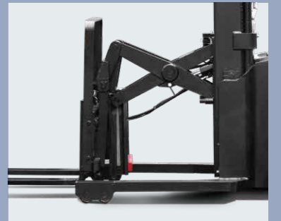
Forks move forward by the scissor structure
